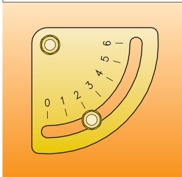
Example of air damper of GI/EMME burners
