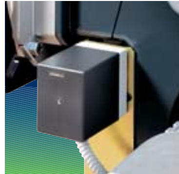
Example of the servomotor for air/oil setting
